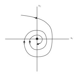
Figure 5.2: Phase plane of (5.20). The origin is a sink.
