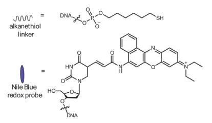
**Figure S3.** DNA modifiers used in this study. The moiety used for self-assembling DNA to the electrode surface is the C6 Thiol Modifier S-S from Glen Research. The Nile Blue redox probe was attached by coupling the dye, Nile Blue A perchlorate, to the NHS Carboxy DT phosphoramidite from Glen Research.
