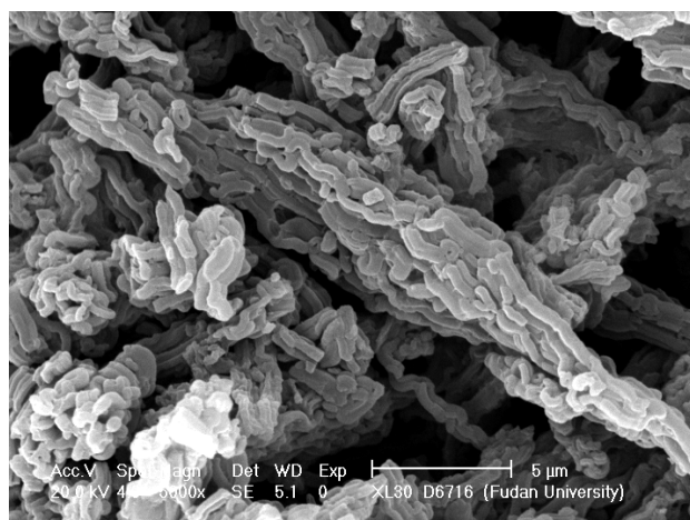
Figure S1. SEM image of ordered mesoporous SBA-15 template.
