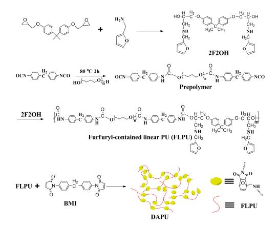
Figure S1. The synthetic procedures of FLPU and DAPU.
