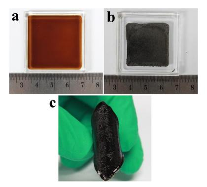
Figure S2. The optical images of GO solutions (a), FAGS (b) and FAGS/DAPU (c).
