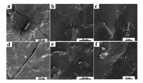
Figure S7. Visual inspection of the healing process of FAGS/DAPU by microwave: (a, d) fissures were cut by a knife, (b-c and e-f) surface of the sample after healing at different magnifications
