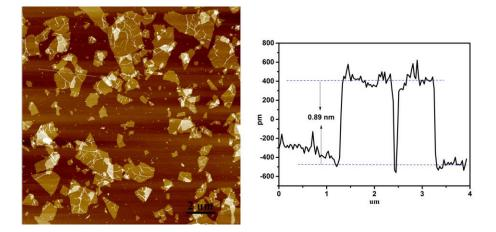
Figure S3. The AFM image of the as-prepared GO sheets.
