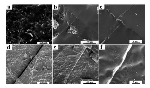
Figure S6. Visual inspection of the healing process of FAGS/DAPU with heat: (a, d) fissures cut by a knife, (b-c and e-f) surface of the sample after healing with heat at different magnifications
