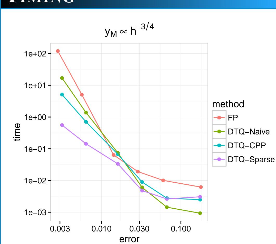
DTQ methods are nearly 100x faster than FP (Fokker-Planck) solver for same level of error. Here we compare three implementation of DTQ:
