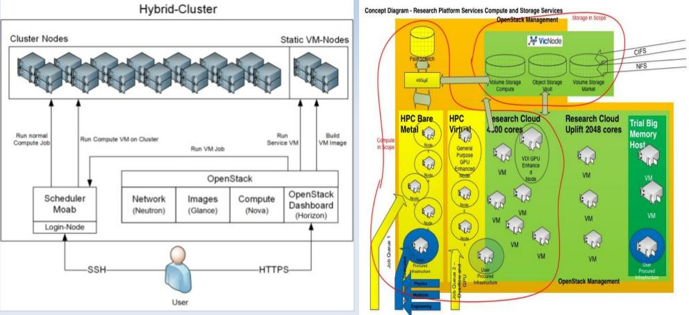
Fig. 3: OpenStack integration and user access
