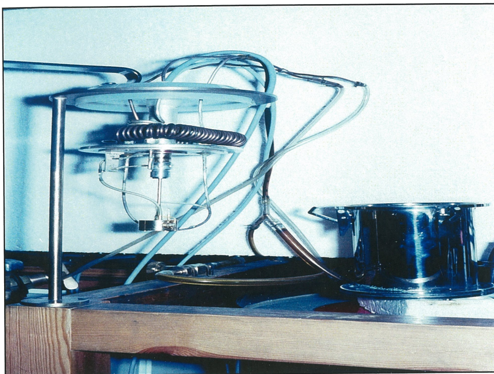
Prototype LKB vapourisation calorimeter, Lund Thermochemical Centre, 1967.
