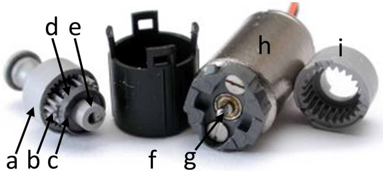
Figure 3.4: GM15 two stage planetary gearbox showing a) gearbox output shaft with top annular gear, b) planet gear, c) pin connecting planet gear and carrier, d) carrier, e) sun gear connecting motor to gearbox, f) shell that holds down output stage, g) motor output shaft, h) GM15 motor, i) bottom annular gear
