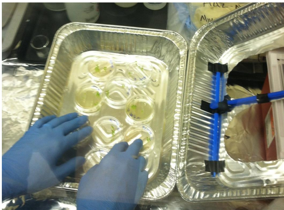
Figure B.1. Duckweed cultures being exposed to NP suspensions in an aluminum tray inside a standard fume hood. Holes in the cover pan on the right are for cool fluorescent lights (not shown). The blue tubes are disposable spatula inserted as structural supports.
