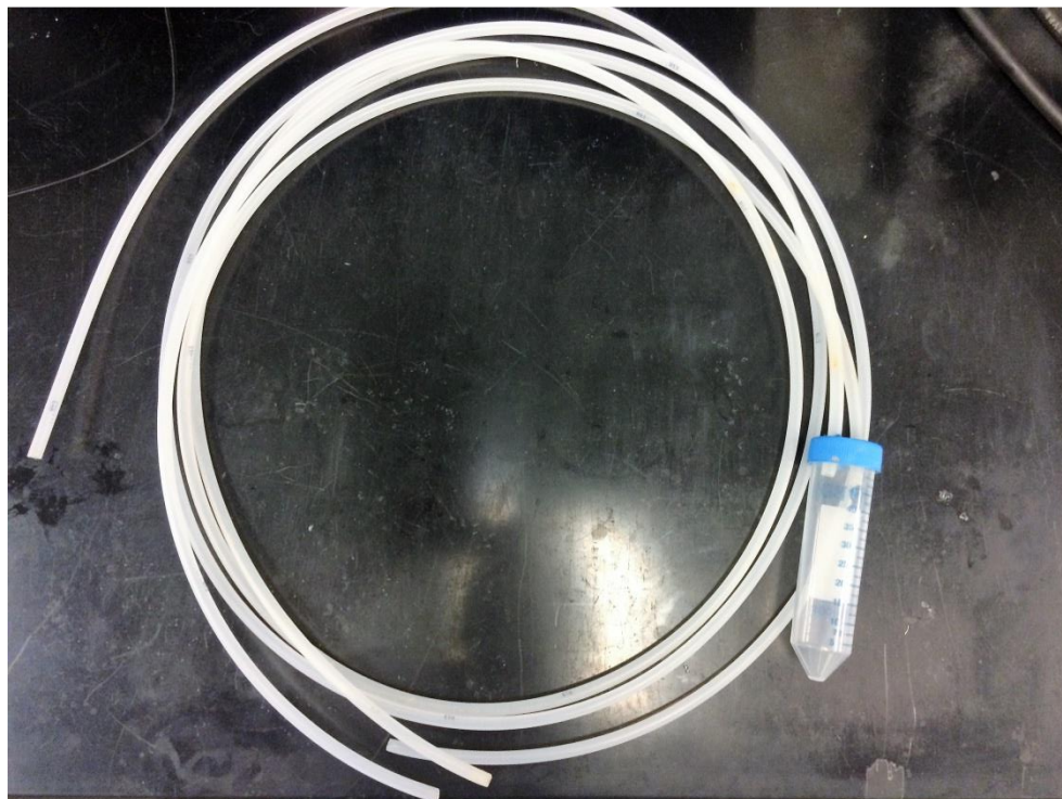
Figure C.1. Image of surficial sampling device using a modified falcon tube and two tubes.
