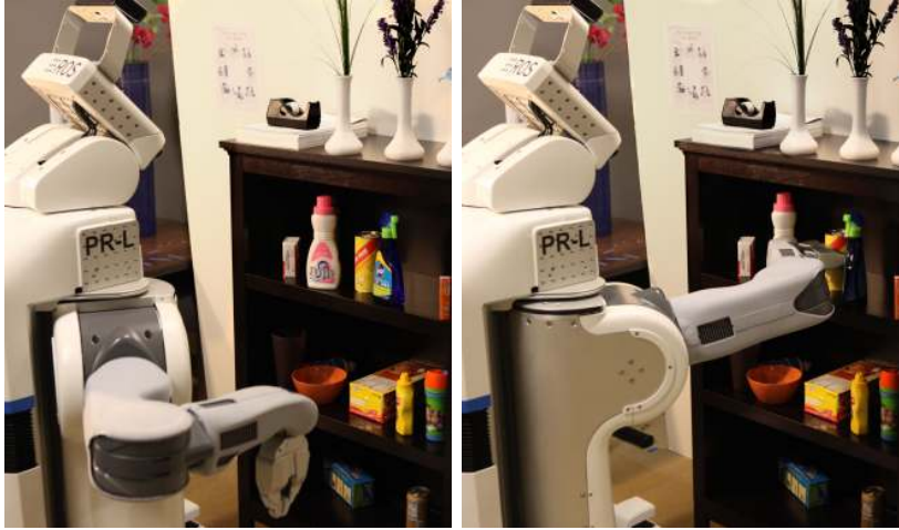
Figure 3.1: Manipulation in a constrained and cluttered environment. Left: a robot tries to acquire a partly occluded object from a constrained shelf space. Right: the robot clears a path to the target by pushing obstacles in a controlled manner, and completes the grasp.
