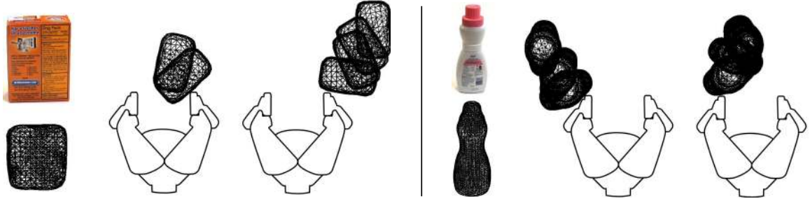
Figure 3.2: Example objects, their trimesh models, and computed trajectories of objects as the hand pushes them. The hand motion is towards the top of the page in each diagram, and is not shown.
