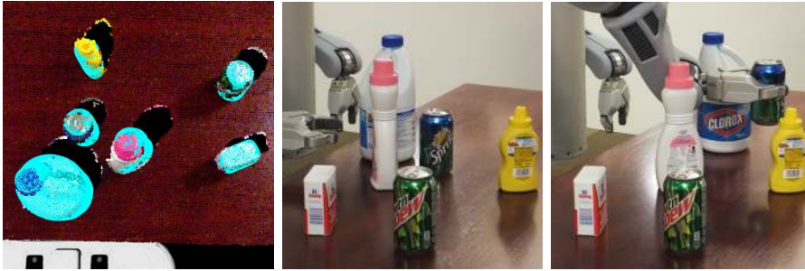
Figure 3.8: An example execution of a randomly-generated scene. Left: Object meshes in the randomly-generated scene configuration, along with point cloud from a Kinect TM camera. Middle: Actual scene with gripper at start of push. Right: Actual scene after object has been grasped.
