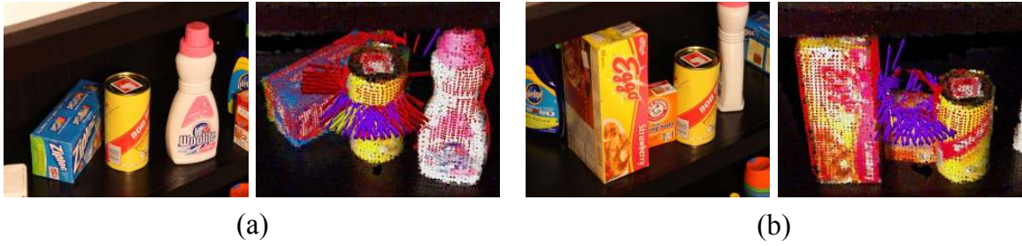
Figure 3.11: Examples of cases where our planner cannot find a solution. In (a), multiple objects start out in contact with each other and object-object interaction during pushing is inevitable. In (b), insufficient space behind the target object prevents the execution of sufficiently long pushes.
