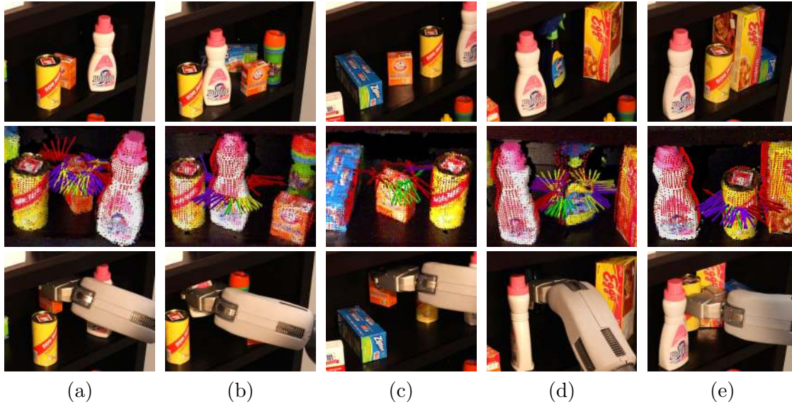
Figure 3.10: A wide range of scenes and objects for which our planner succeeds by moving obstacles in a controlled manner. Each column shows one grasping task. For each column, top image : Initial scene; middle image : Scene as seen by the robot, showing an acquired point cloud superimposed with object recognition results (red point object outlines) and evaluated grasping directions (arrows); bottom image : Final result of successful grasp execution.
