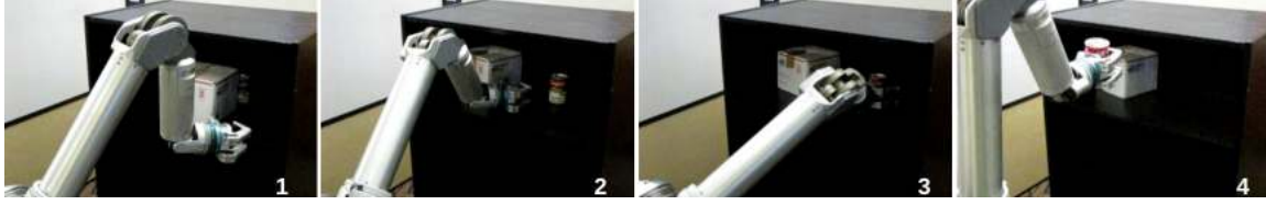
Figure 4.7: An example plan to retrieve a can hidden behind a large box on a shelf. The pick-and-place planner fails to find a plan in this scene. But pushing planner finds the presented plan. Planning time is 51.2 sec.
