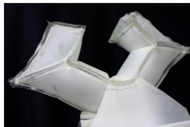
(c) Inflatable hand - closed state
