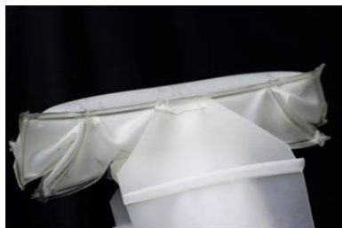
(b) Inflatable hand - open state
