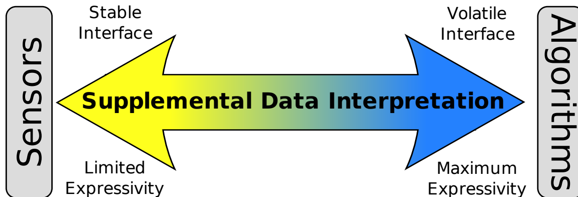
Figure 5.5: The critical tradeoffs a designer must make when choosing to keep interpretation “close to the sensors” vs. “close to the consuming algorithms”.
