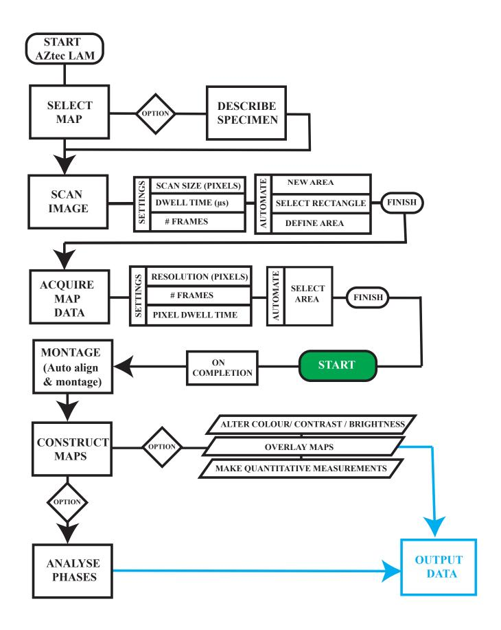
**Fig. S2.** Flow chart of typical workflow for the acquisition of AZtec LAM (Oxford Instruments) EDX map montages. Blue represents output of data for external manipulation. Basic acquisition illustrated, additional options not shown.
