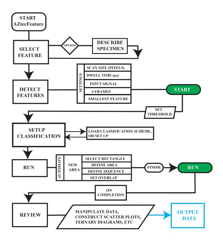
**Fig. S3.** Flow chart of typical workflow for the acquisition of AZtecFeature (Oxford Instruments) particle analysis. Blue represents output of data for external manipulation. Basic acquisition illustrated, additional options not shown.
