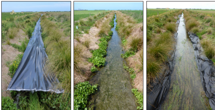
Suspended polythene (left), handweeding (center), and weed mat (right) treatments extend over 50m reaches in a Hinds waterway.
