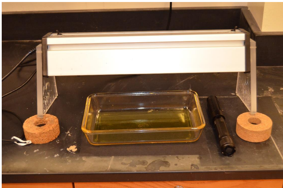
Figure S49. The set-up of writing in solution. The glass container was placed beneath the 365 nm UV lamp, which was set up to excite 1 so it will emit fluorescence, and subsequently isomerize thus erasing the writing.
