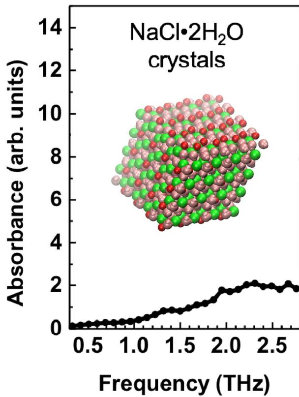
Figure S2. Calculated THz absorption spectrum of sodium chloride dihydrate crystals.
