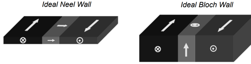
Figure 2.6: Ideal Bloch Wall and ideal Néel Wall Transitions.
