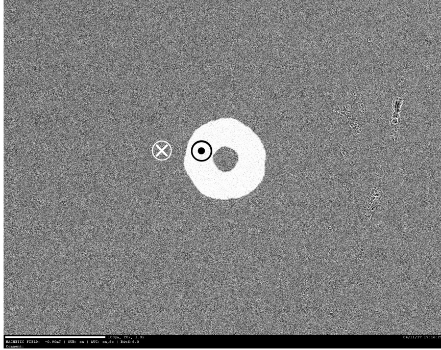
Figure 5.10: Example MOKE image of a bubble domain for Pt-Ir alloy seedlayer films.
