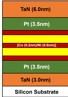
Figure 6.1: Symmetric multilayer with Pt/Co and Co/Pt interfaces.
