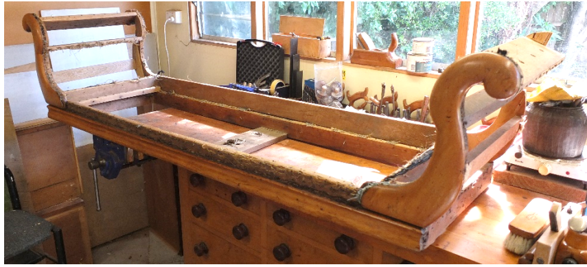
FIG. 1 Rimu and kauri neo-Grecian sofa, with turned legs, backrest and upholstery removed. Note the traditional glue pot on the far right.
