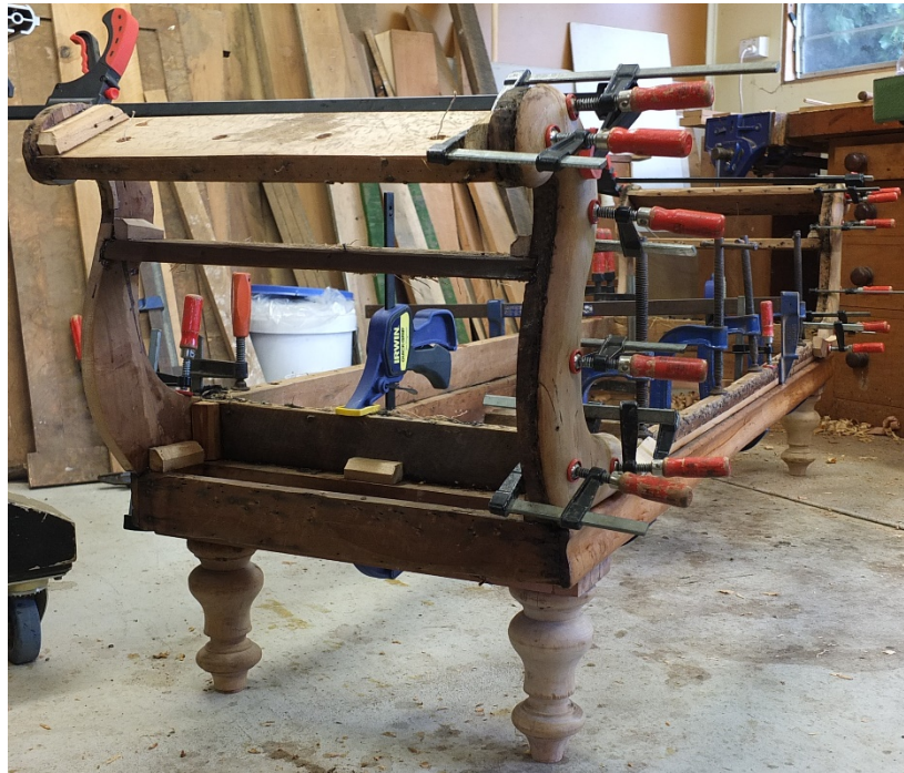
FIG 10: Sofa clamped after reassembly with gelatine glue.
