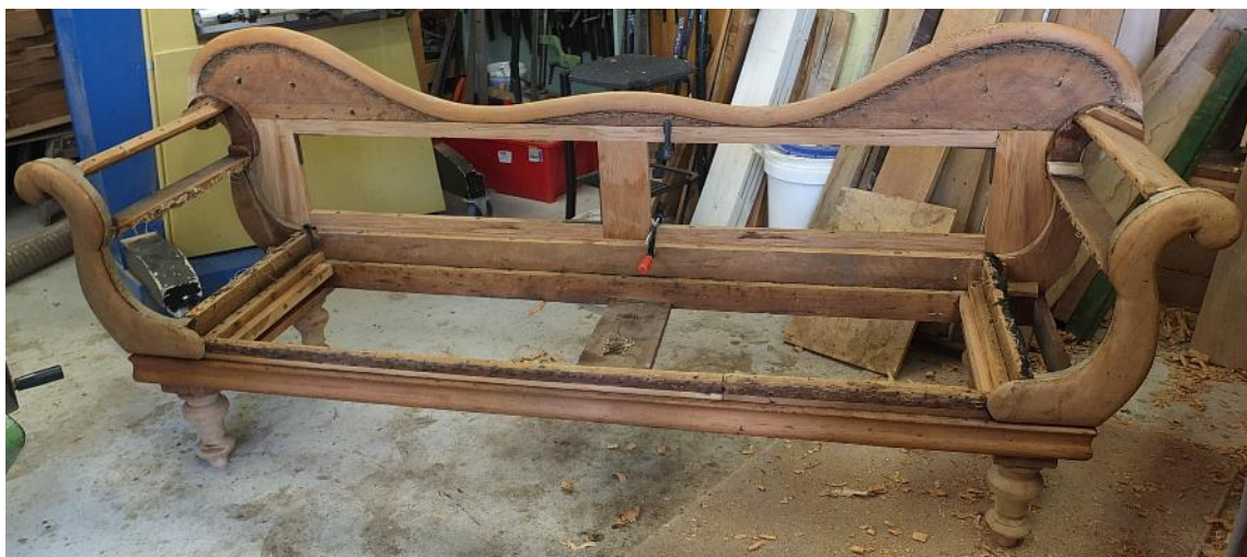
FIG 11: Sofa with all wood repairs finished. While the new rimu can be seen in the backrest replacing a makeshift repair particle board panel, there is little other evidence to suggest such invasive work had ever been undertaken.
