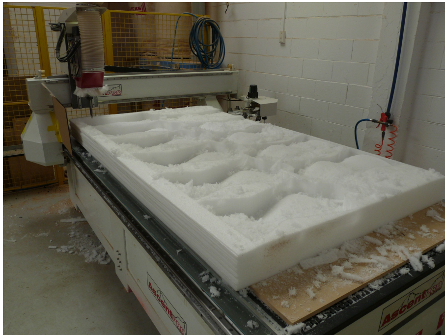
FIG. 4: The Ethafoam forms being milled by the CNC router at the Te Mahi workshop.
