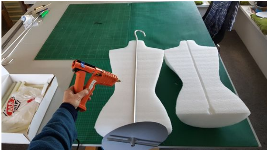
FIG. 5: Tubular aluminium hanging hardware being inserted into the forms at the Triptych workshop.
