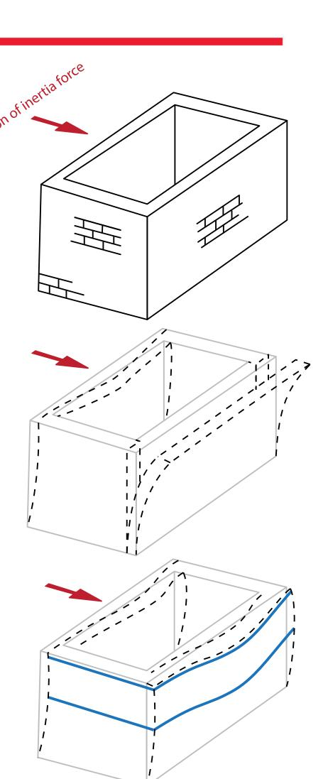
Structure under loading without and with seismic bands (adapted from Caon 2009)
