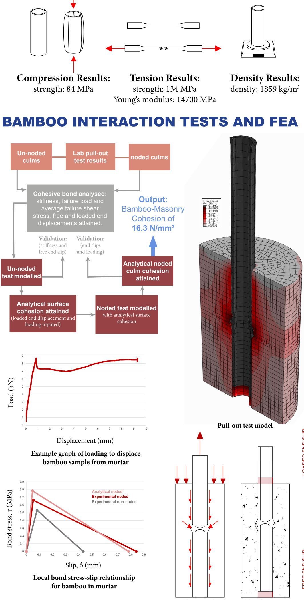
Pull-out test loading and displacements
