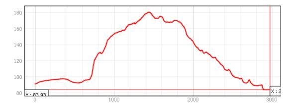
Since the elevation model is measured in metres, the vertical and horizontal scales are in metres. The vertical is given as m a.s.l. (metre above sea level; the elevation) whereas the horizontal is given as metres from the starting point.
