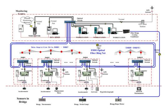
FIGURE 6.4: The network topology of bridge structure health
