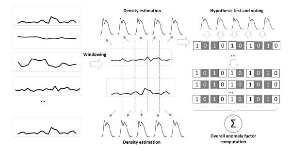
FIGURE 5.1: Procedures of Multi-dimensional Ensemble Kernel
