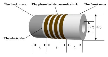
FIGURE 2.2: Example of a PTZ sensor
