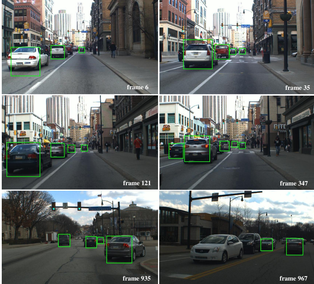
Figure 4.6: Qualitative multi-object tracking results on our vehicle data set.
