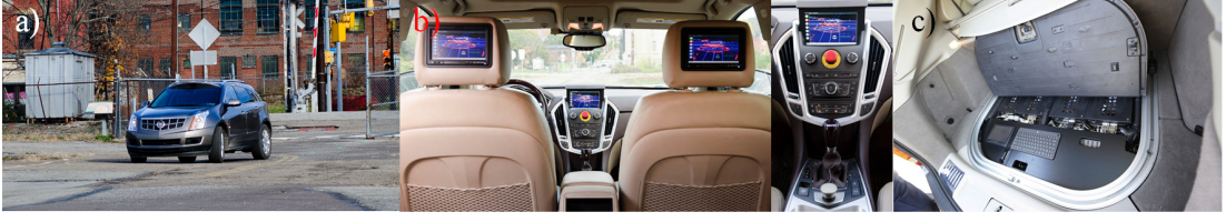
Figure 5.7: Our experimental vehicle and its sub-components. (a) Autonomous Cadillac SRX [109], (b) Display and control console, (c) Computing cluster.
