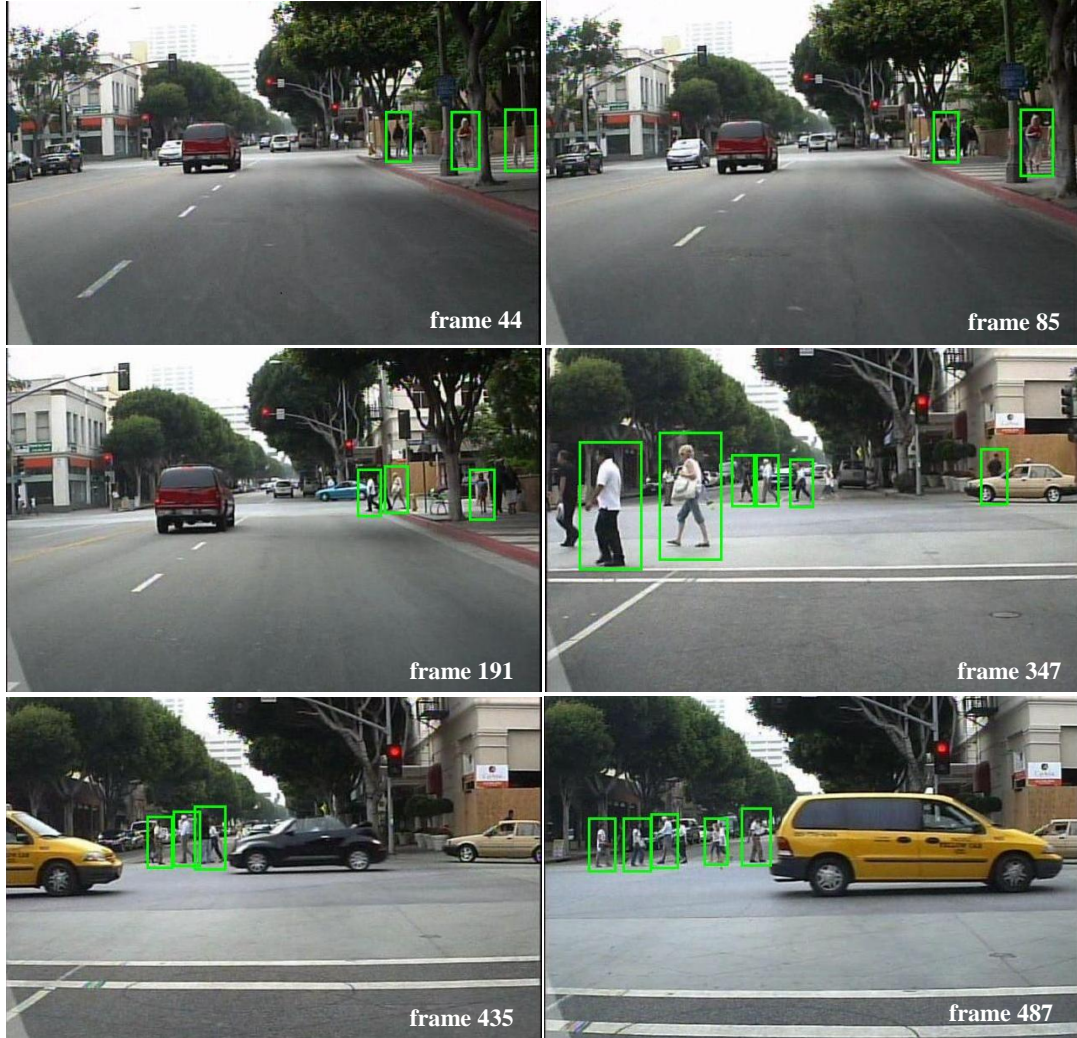
Figure 4.5: Qualitative multi-object tracking results on the Caltech test set.
