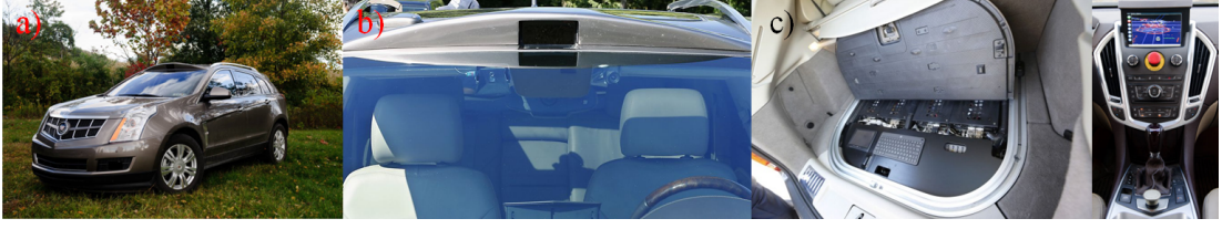
Figure 3.10: Our experimental vehicle and its sub-components. (a) Autonomous Cadillac SRX [109], (b) Forward-looking camera (monocular setup), (c) Computing cluster and control console.
