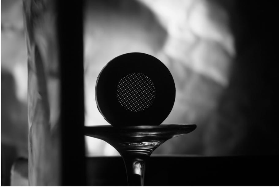
**Figure 2.8:** Uniformly illuminated pin-hole grid used in our experiment to measure the response of pixels behind the Bayer array of the camera sensor, to different wavelengths
