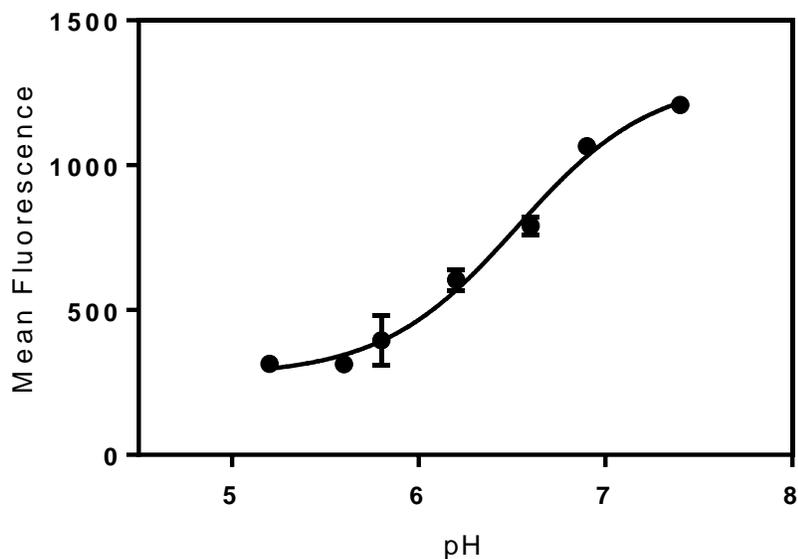
**Figure S-2.** Binding of aptamer S8 to 50 nM SA-PE over a range of pH values. Half-maximal binding occurs at pH 6.5. The mean  $\pm$  standard deviation for three experimental replicates is shown for each pH.
