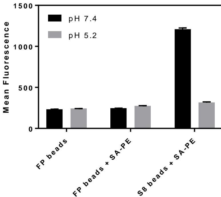
**Figure S-1.** Forward primer (FP)-coated beads show no difference in fluorescence in pH 7.4 and pH 5.2 selection buffer, either with or without 50 nM streptavidin-phycoerythrin (SA-PE). The mean + standard deviation for three experimental replicates is shown for each sample.
