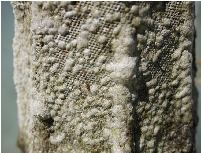
Figure 11. mineral accretion test produced in Kelonia (turtle research centre) in La Réunion Island 2017. Photos: David Enon
