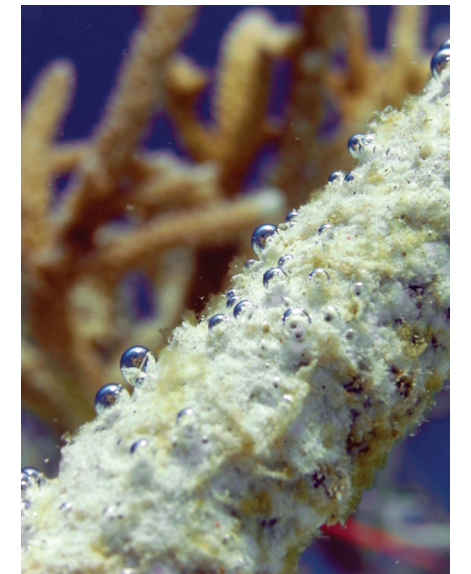
Figure 4. Small hydrogen bubbles form around the structure of a Biorock artificial reef under construction. They testify to the proper functioning of the mineral accretion device. Photo: Foued Kadhachi
