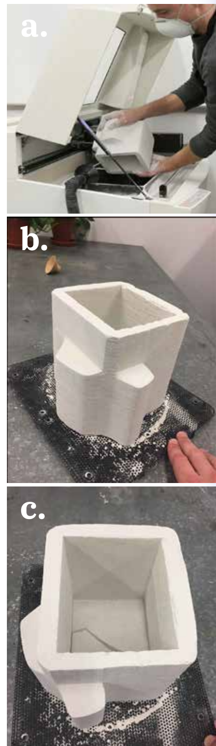
Figure 13. 3D printed moulds for glass casting, pre-firing.
