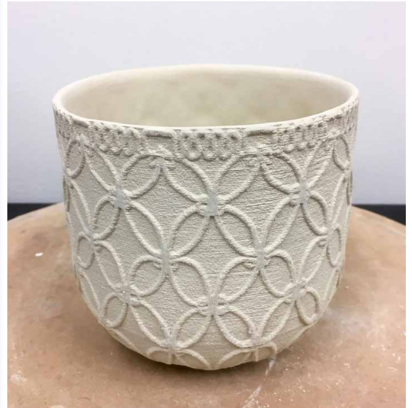
Figure 11. Cast porcelain cup from 3D printed mould.
