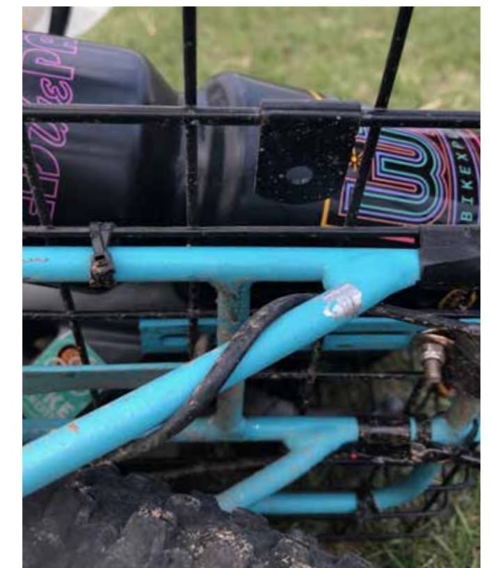
Figure 7. Site of repair: A cracked and bent front rack caused rubbing on the tire, Rep(AIR) diffused cinnamon to communicate the impact.
