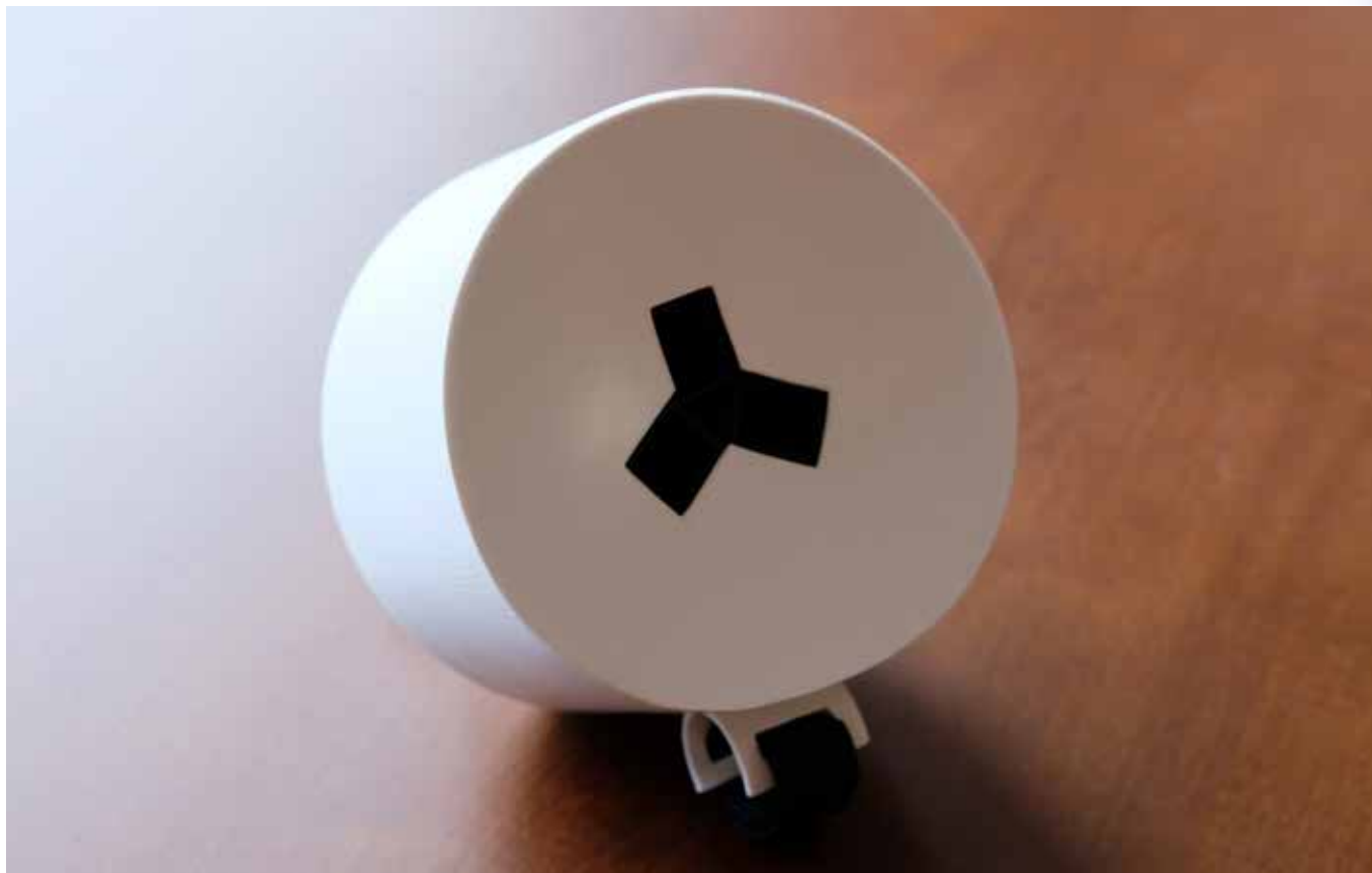
Figure 5. Housing: Sheets of white polystyrene were vacuum molded, hand molded, and textured creating a clean bright outward appearance. The hand cut lid was meant to abstractly resemble a flower.
