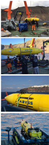
Fig. 2. AUV-Abyss (GEOMAR) operations on board R/V POSEIDON (March 2017) (photo credits to Sven Petersen).
