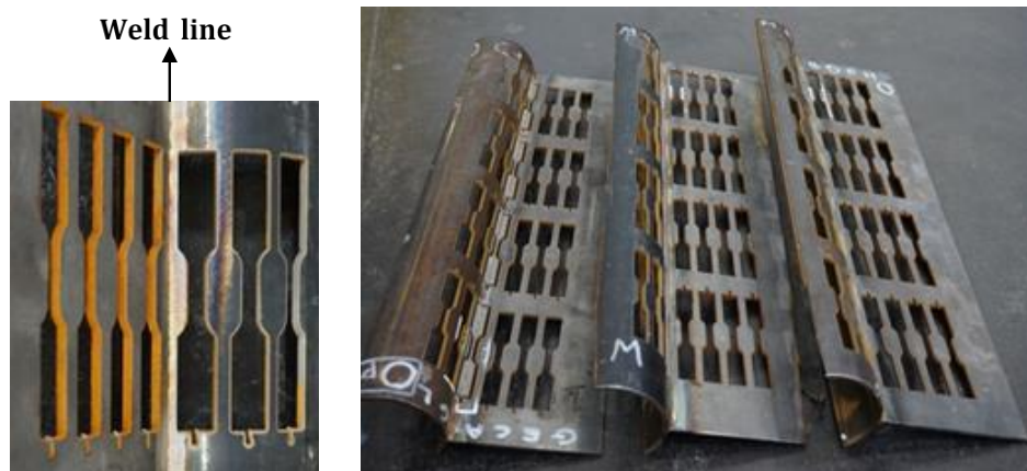
Figure 3.4. Tensile specimens extracted from the sample section.
