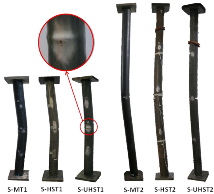
Figure 4.4. Failure mechanism comparison of one and two-meter single MT, HST and UHST specimens
