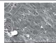
Figure 4: SEM micrograph of bacterial cellulose grown in a medium containing PHB.
