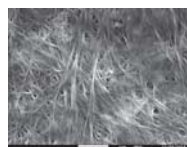
Figure 1: SEM micrograph of bacterial cellulose without any additives in the medium.
