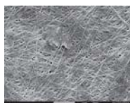
Figure 2: SEM micrograph of bacterial cellulose grown in a medium containing HPMC.
