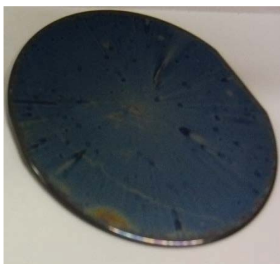
Figure 2: Appearance of cellulose films made from cellulose nanocrystals aqueous dispersion (6.5 wt %) on silicon wafer (diameter=50.8 mm).
