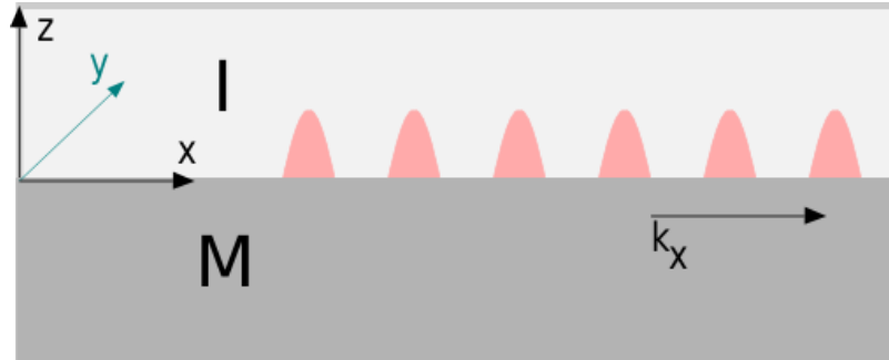
FIGURE 3.6: Geometry of simple plasmonic waveguide with wave propagation along the x direction and homogeneity in y such that \partial/\partial y \equiv 0 .
