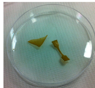
Figure 8. Films prepared from dissolved feather in [DMEA][HCOO].
