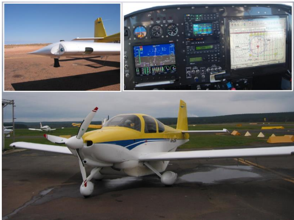
Figure 3.2: Experimental aircraft showing a wingtip installation in the left inset, and the cockpit with cockpit computer display in the right inset (Walker et al., 2009).
