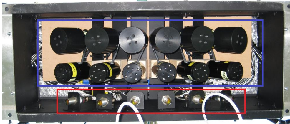
Figure 3.5: Sensor box with 12 multi-spectral radiometers (two upper rows indicated by blue box) and 6 thermal infrared radiometers (bottom row indicated by red box) (Walker et al., 2009).
