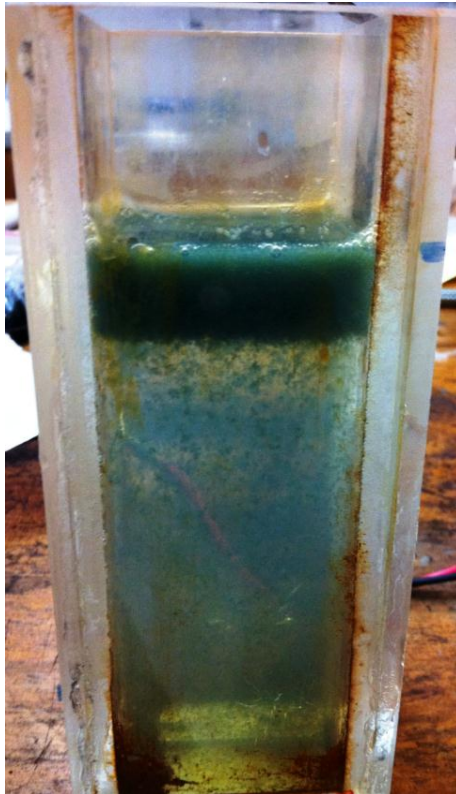
Figure 5. 13. Electrocoagulation performed on salt water media at 5 V, with the stainless steel 430 anode.
