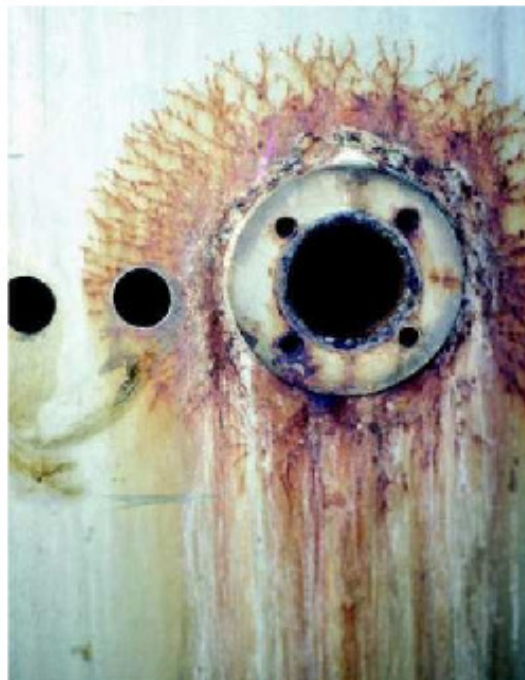
Fig. 2.5 SCC in stainless steel used for food processing vessel (Elliott, 2003).
