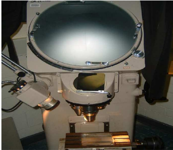
Fig. 3.9 Profile projector used to measure crack size (Pal, 2010).
