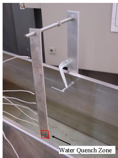
Figure 3-1 Sample with embedded thermocouples in the quench rig designed by Sweet et al. [8].
