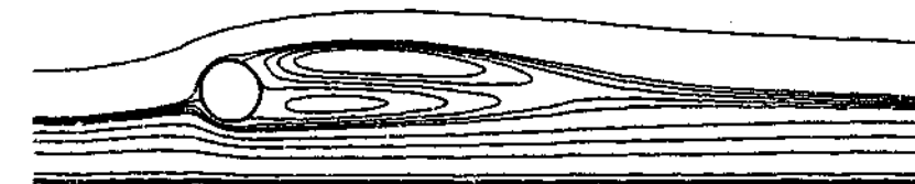
FIGURE 3.3: Flow streamlines around a ring with aspect ratio Ar = 3 at Re = 100 , following the separation transition, illustrating the recirculating region behind the ring cross-section. Arbitrary contour levels are used to highlight the flow structures.
