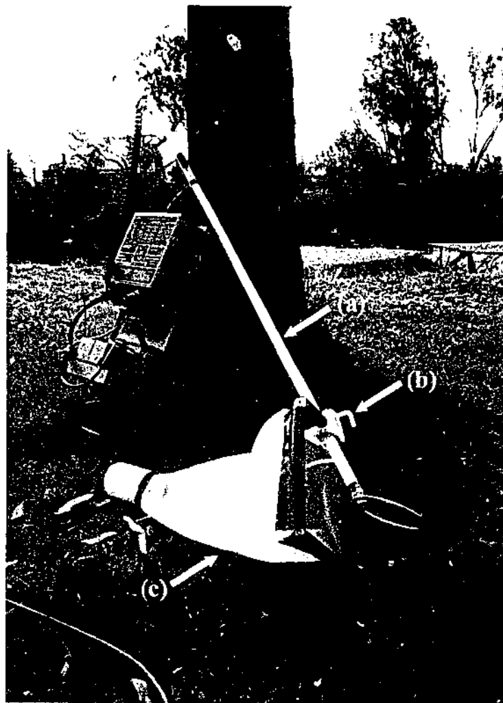
Figure 3.1: Modifications made to a standard backpack electrofishing unit for the SNE method. (a) Anode pole with attached 15 cm diameter anode, (b) plastic formed screw and frame, (c) Nylon material with velcro lining for attaching 250 \mu m mesh net to plastic frame.
