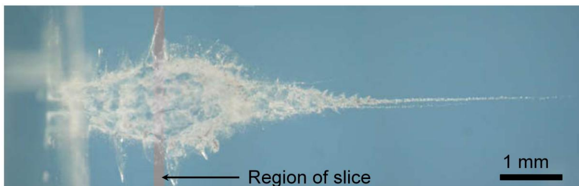
FIG 5.1: Track #41. This is a Type B track of length ~4 mm and the impact was from the left of the image moving right. It was removed from the cometary collector cell 44. Our slice was cut 0.8 mm in (grey vertical rectangle) from the track entrance. Track image courtesy of NASA-JSC.
