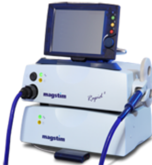
Figure 2-3 Example of a modern transcranial magnetic stimulator
