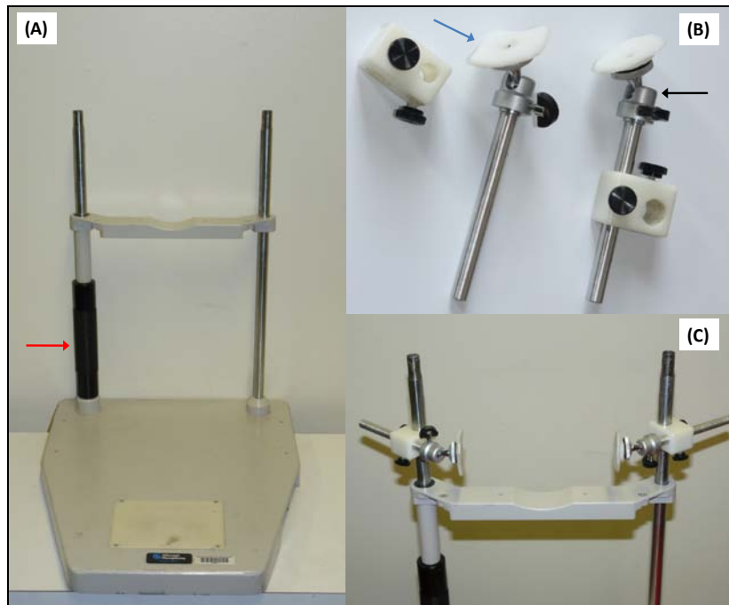
Figure 2.15: Chin rest (A) and cheek supports (B) used for head stabilisation. The handle on the chin rest (red arrow) enabled the patient to adjust the height of the chin rest to a level comfortable for the subject. The cheek supports were designed and partly made by the author and Dr. Proudlock, the material at the end of the cheek support (blue arrow) was made using Rolyan® Aquaplast®. Once this material is immersed in hot water it becomes transparent and soft, it is then moulded into the desired shape and allowed to cool. The remainder structures were made by the engineers at the medical physics workshop. The ball joint (black arrow) allowed control over the cheek supports to accommodate different facial contours. The final picture (C) shows the cheek supports mounted on the chin rest.
