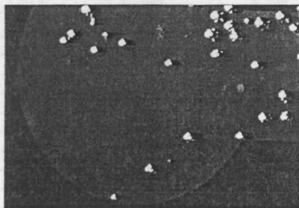
Figure 4.15 Bitmap image of the vertical gold electrode showing distribution of nucleation sites over the surface. The electrolyte was 0.1M HClO 4 . Gas was evolved at 2.8 mAcm -2
