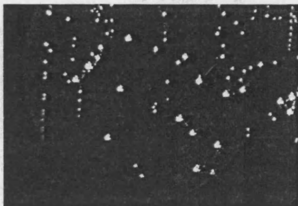
Figure 4.21 Bitmap image of the vertical gold electrode showing distribution of nucleation sites over the surface. The electrolyte was 0.1 \text{ M HClO}_4 . Gas was evolved at 44 \text{ mA cm}^{-2} .
