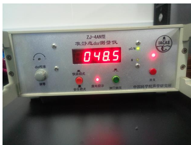
Figure S6. Photo of the piezoelectric coefficient d_{33} of 1 measured along c -axis at room temperature.
