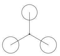
Figure 5.2: Tuning machine with changing angle. The 3 circles in the figure are nozzles and can rotate around itself. The angle between the arms is constant and 120 degrees. The arms can approach each other like joining the fingertips to reduce or enlarge the diameter.
