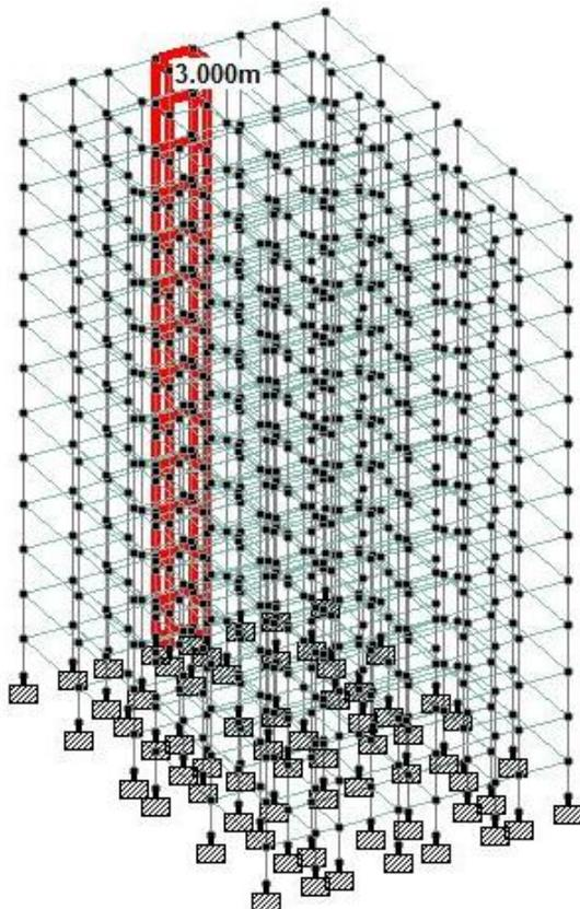
Fig. 3: Building B1 Flat Slab with Shear Wall
