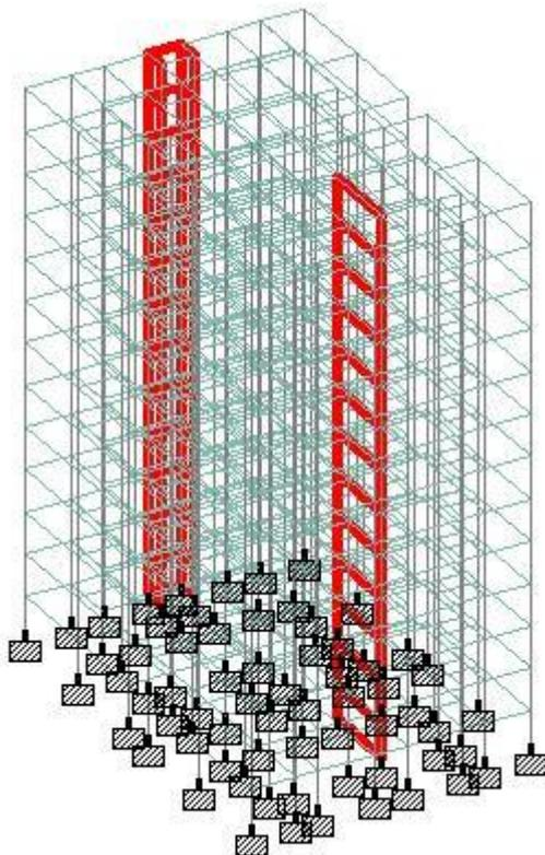
Fig. 4: Building B1 Flat Slab with Shear Wall at Maximum Stress Location
