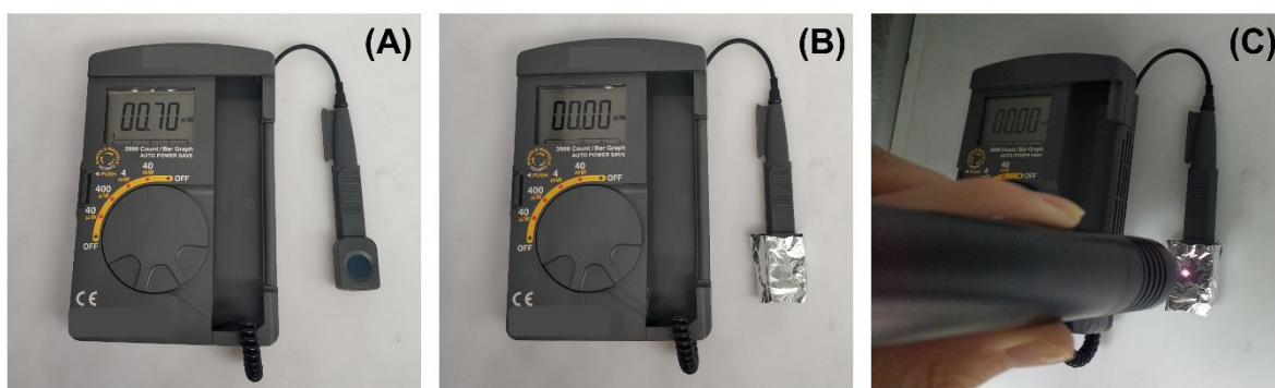
Figure S9. Photos of the laser power meter under (A) electric light environment without foil wrapping, (B) electric light environment with foil wrapping, (C) NIR laser with foil wrapping.
