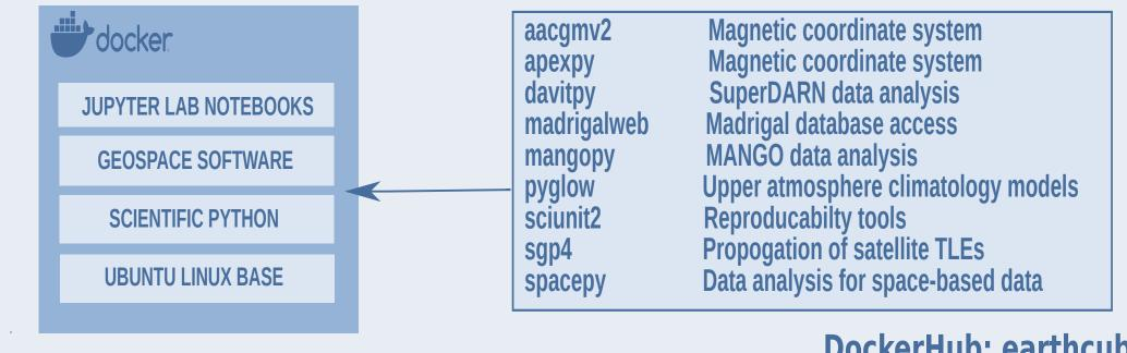
The resen-core Docker image builds upon a standard Ubuntu Linux image and comes pre-installed with a stack of commonly used geospace libraries and software packages. This approach allows users to avoid the arduous and often time-consuming task of manually installing software on their local systems and provides a consistent platform for collaboration and reproducibility. New releases are made twice a year to incorporate newer versions of the packages. The releases are available on DockerHub.
