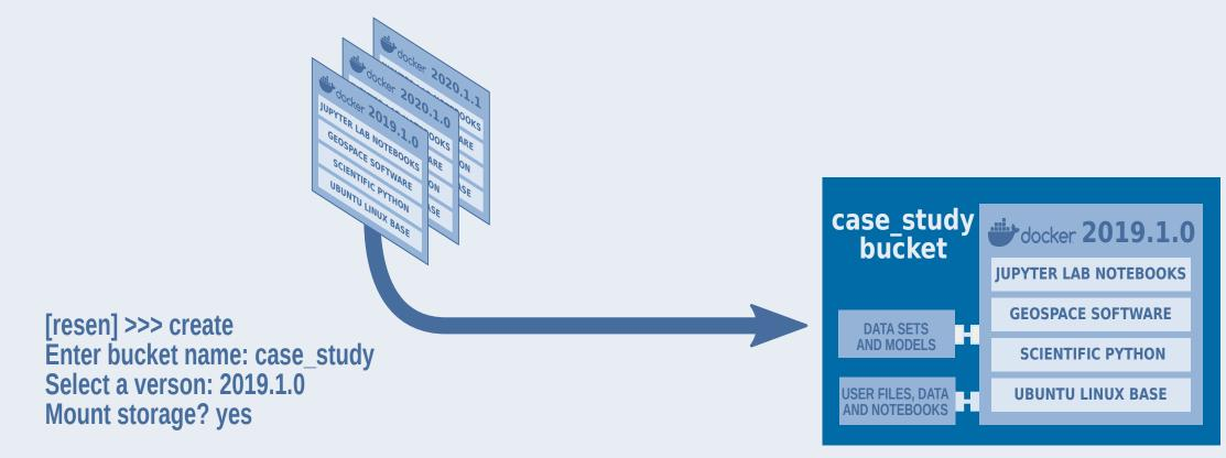
Within Resen, data analysis environments are called buckets, consisting of a Docker image and mounted file volumes where a user's files will be stored. In addition, there is a mount for common data sets and models. The resen create command is used to make a new bucket, which is based on one of the available resen-core images.
